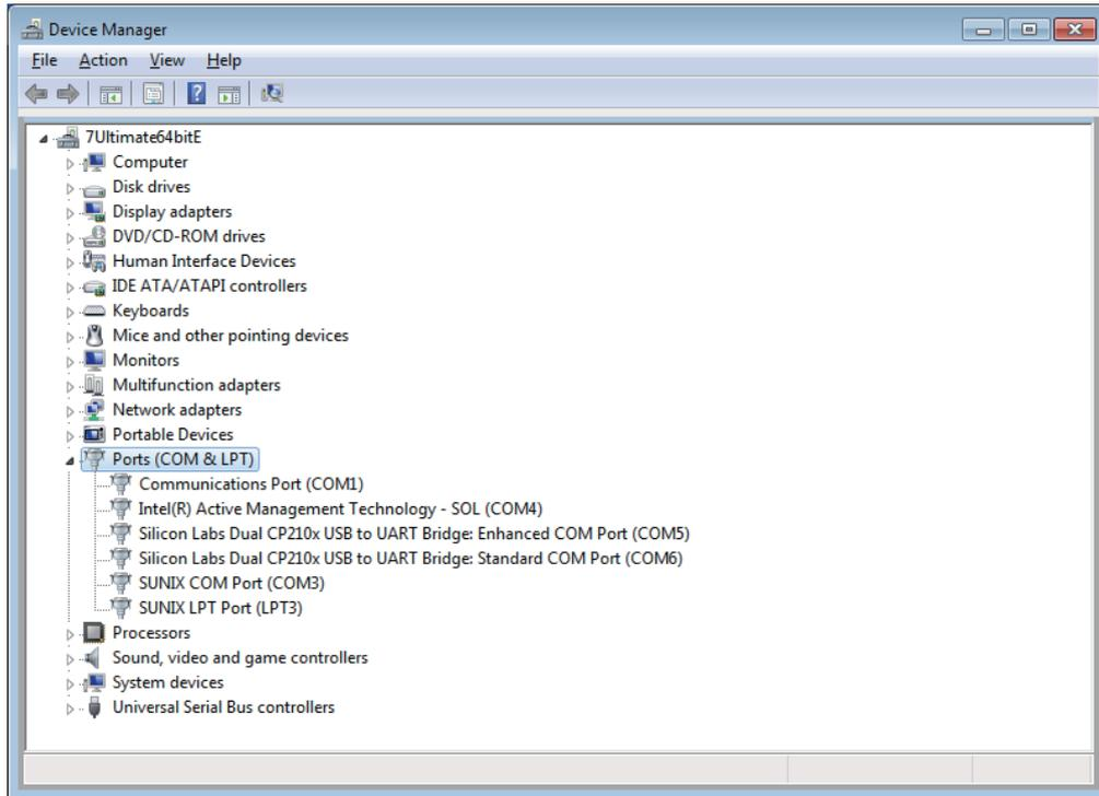
SCU-17 contain two virtual COM ports, an Enhanced COM Port and a Standard COM Port. These ports offer the following functions.
